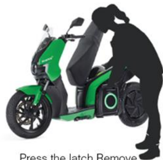
Press the latch Remove the battery pack
